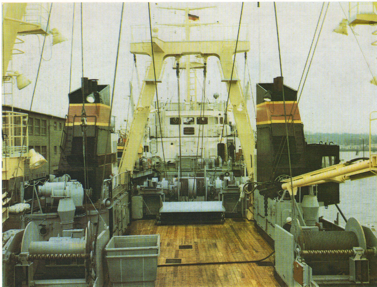
Catch deck with trawl warp winches and multi-drum auxiliary winch
