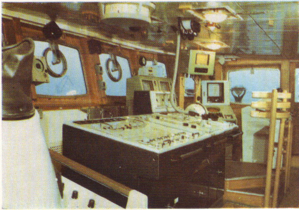
Forward part of bridge with bridge control stand, radar and fish locating installations
